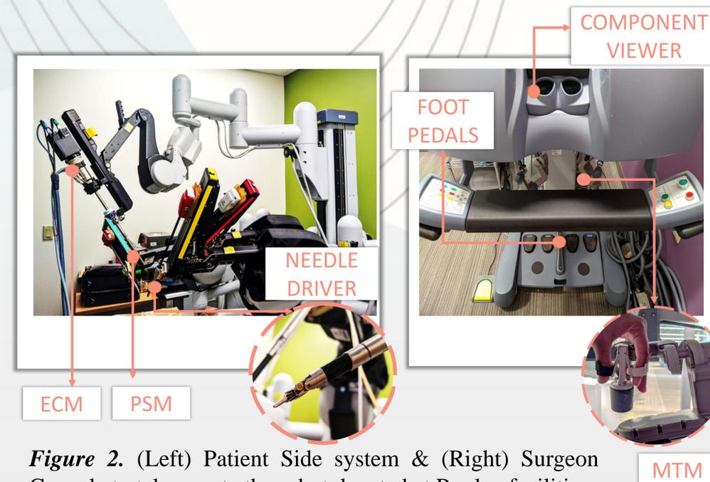
Figure 2. (Left) Patient Side system & (Right) Surgeon Console to teleoperate the robot, located at Purdue facilities.
