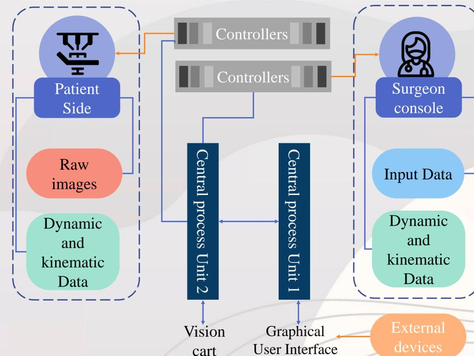
Figure 3. Interaction between components from the general system and data obtained as a result from teleoperation of the robot.
